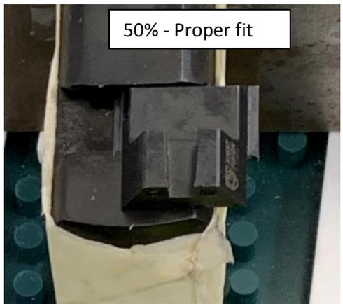
\*\*Forcing a gun sight that does not fit properly with gunsmith tools can and will damage the gun sights. This is considered an improper installation and is not covered by warranty.
