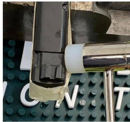
\*\*If gun sight does NOT move with ease, most likely not enough material was removed in step 6, and that step should be performed again until fitted properly.
