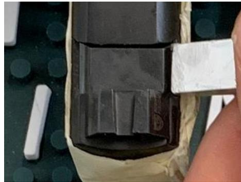
**\*\*Striking the blade with Drift or Hammer during installation and causing any damage to the sight or tritium lamps will not be covered by warranty.**
