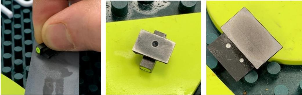
\*\*It is important to frequently check and test fit the gunsight. Removing too much at one time can cause the sight to be too loose. This is considered an improper installation and is not covered by warranty.
