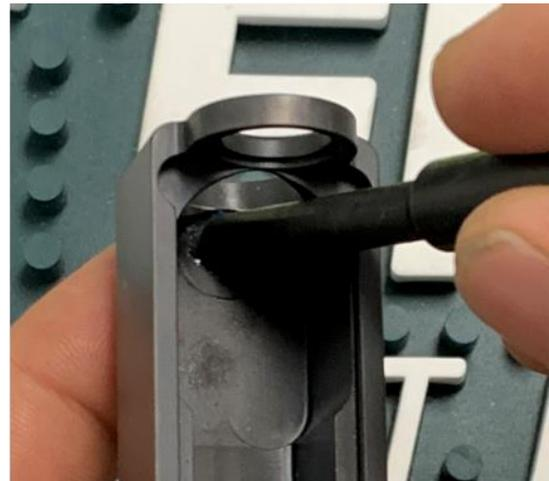
7. Once the front sight is in place, clean off excess Blue Loctite using a Q-tip and cleaner and allow loctite to set over night.
