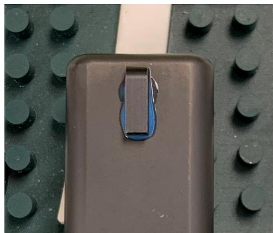
6. Holding the front sight in place with one hand, flip the slide upside-down and insert the provided Night Fision screw into the boss using a 3/16<sup>th</sup> hex driver. Tighten hand tight 5-7 in-lbs. of torque. Only tighten securely after double checking the sight alignment is centered.
