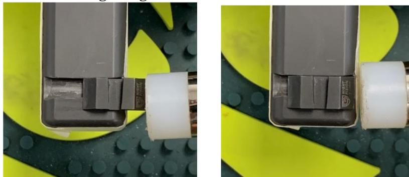
\*\*If gun sight does NOT move with ease, not enough material was removed in step 10, and that step should be performed again.
