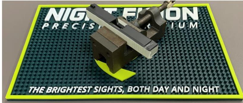
9. **Test fitting gun sights:** Insert gun sights into the slide dovetail by hand, using firm pressure until stopped.
